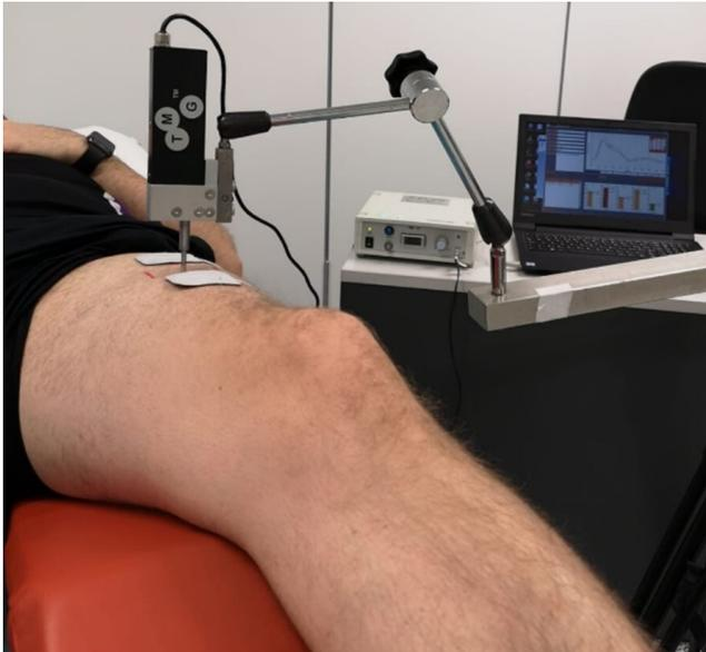
**Figure 2. Equipment set up during TMG assessment of the RF muscle**
